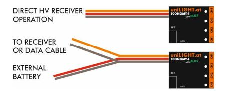
In the uniLIGHT system, lights can easily be switched in parallel. Therefore, four functions are sufficient for most applications. Connections can be made using a Y-cable or simply by soldering together. With the Economy 4, no more than 3-4 luminaires of the 040 type should be operated in parallel on one channel.
