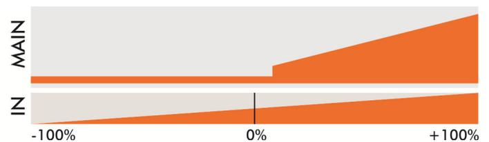
**MODE 3** Output is autonomous generated when a step value is exceeded, the control can be connected parallel to the gas servo. A random stuttering effect is generated which automatically becomes stronger. The switch point can be set via the button in a meaningful range (approx. 20% to 80%).
