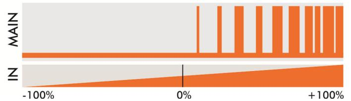
**MODE 2** Output is directly dependent on servo input, direct mode. An increasing glow is generated as output signal.
