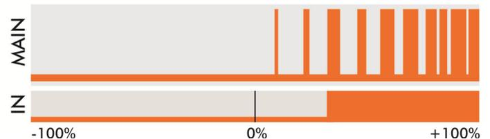
**MODE 4** Output is autonomous generated when a step value is exceeded, the control can be connected parallel to the gas servo. An increasing glow effect is generated.
