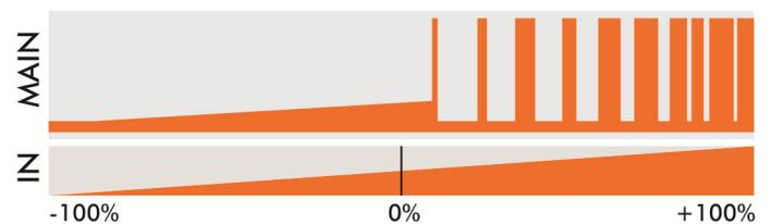
**OPTION 4** In main operation area, a basic continuous basic glow is integrated under the stutter signal. This significantly increases the light output and weakens the hard stuttering. The on-time of the LEDs increases and thus also the temperature. The basic setting is OFF.
