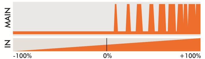
**OPTION 3** A slight, ascending glowing is generated in the region of the lower throttle. The on-time of the LEDs increases and thus also the temperature. The basic setting is OFF.
