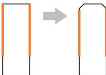
To improve movement and live time it is optional to bevel the contact blade with a file...
