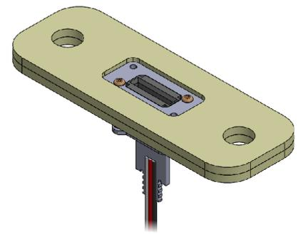
6. Place the supplied template on the plug or fix it slightly with a double-sided adhesive tape.
